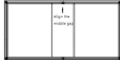
13. Pre-install all leaf springs and nuts from the inside of the inner frame to the corresponding holes. According to the order of the short side first and then the long side, the two persons tighten the nuts synchronously until they are tight.
