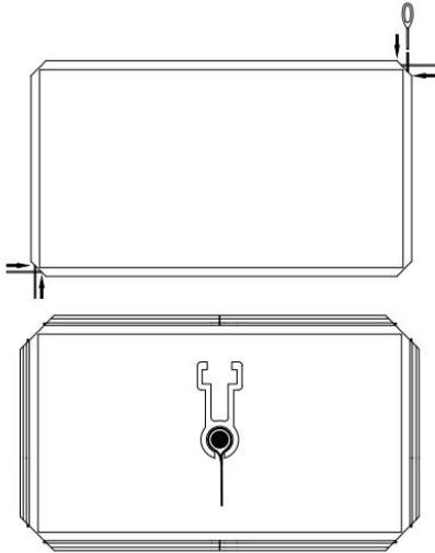
10. The pair lift the inner frame horizontally and put it on the screen base fabric, adjust the position of the inner frame to make it centered.
