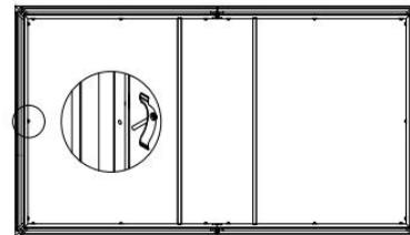
14. Splice the long sides of the outer frame with Outer frame Splice Joint and fix them with screws (m4×6).
