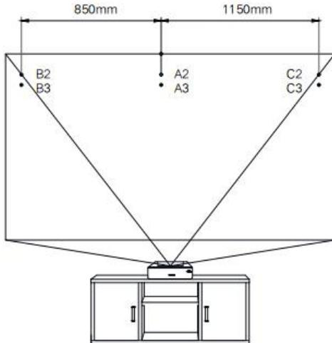
4. Use a drill bit to drill holes at the 6 drilling points. The drill bit diameter is required to be 8mm, and the drilling depth is not less than 65mm.
