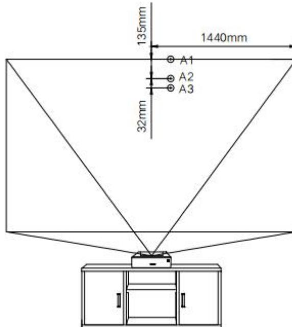
3. Based on A2 and A3, mark and drill holes at 850mm to the left B2 and B3, and mark and drill holes at 1150mm to the right C2 and C3.
