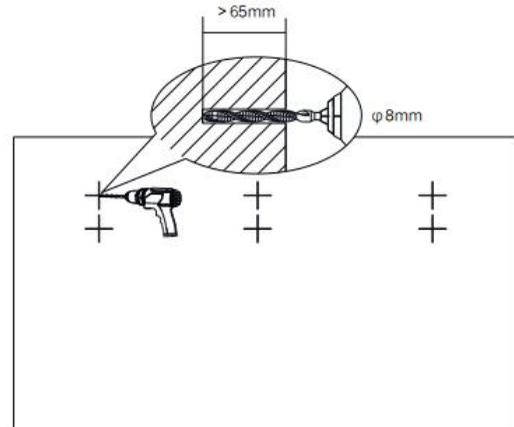
5. Install the expansion screws, pass the expansion screws through the fifth and ninth holes on the wall hanging, and fix the wall hanging on the wall.
