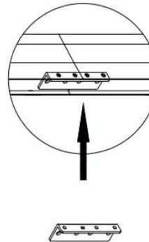
2. Splice the Elbow Joints (inner frame) and the inner frame, use (M4\*6) screws to fix the two outer screws of the Elbow Joints (inner frame).
