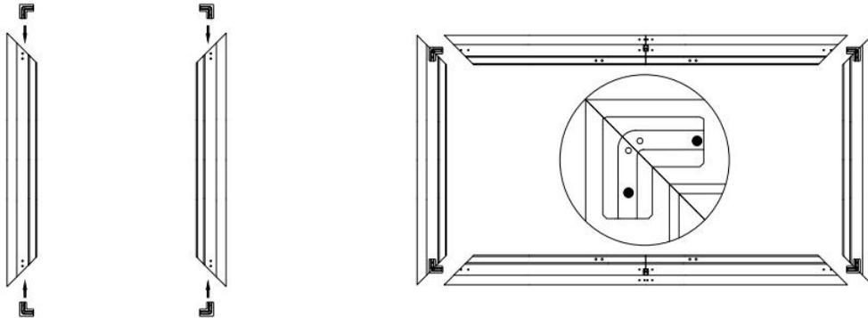
3.Align outer frame four-corner support joint with the threaded holes of Elbow Joints (inner frame) and fix the two screws in the middle of the Elbow Joints (inner frame) with (M4\*6) screws.
