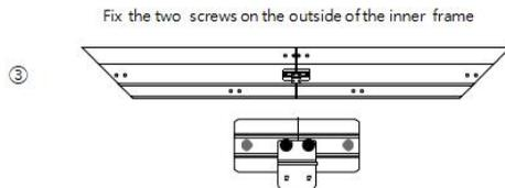
Align the outer frame middle support joint with the inner frame splice joints threaded holes.
